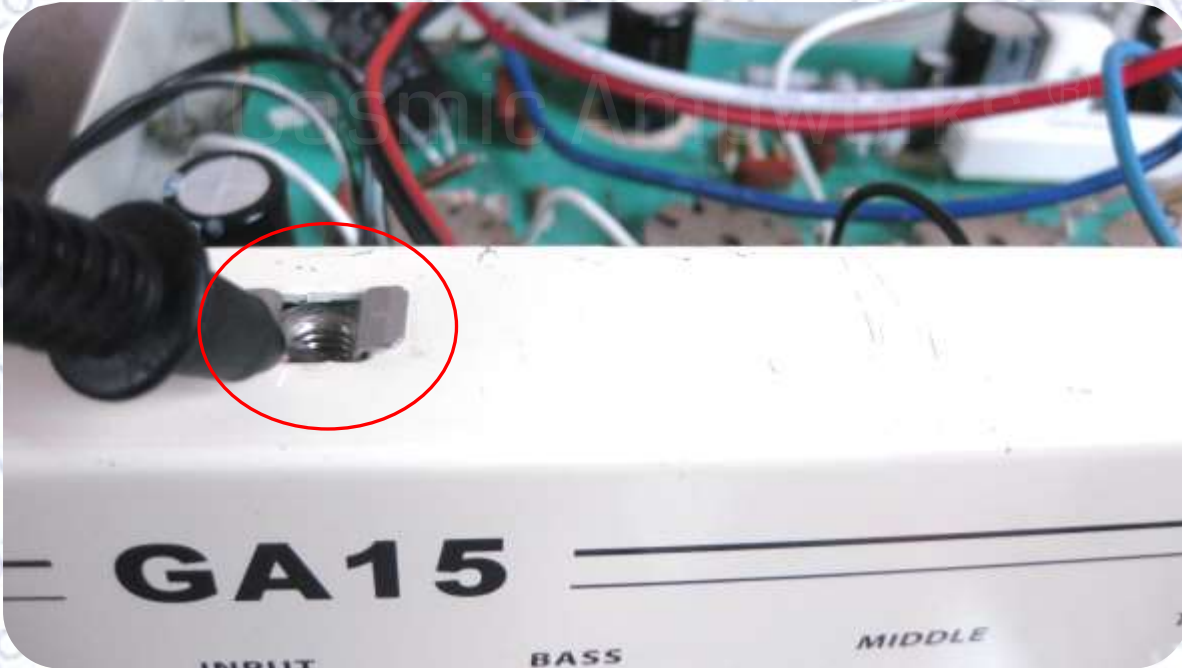
Figure 3. If your multimeter does not have a clip-on ground probe, a (less advisable) alternative is to hang the negative terminal in one of the cage nuts (after switching off and disconnecting the amp), so you can keep one hand free for safety and take measurements with the other hand.
