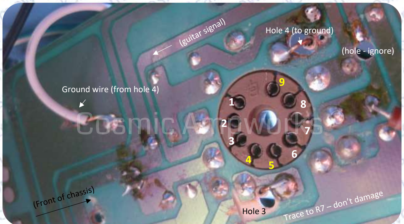
Figure 23. Drill two holes near the first preamp tube: Drill hole 3 right next to the tube socket solder connections of pins 4 and 5; make sure not to damage the trace running from pin 6 of the tube (anode) to R7 (load resistor). Drill hole 4 just above the tube socket solder connections of pin 9. Make sure not to accidentally damage the wire bridge on top of the board! Ideally, also interrupt the circuit board trace in go, because the heater traces spread hum throughout the circuit in their stock layout.
