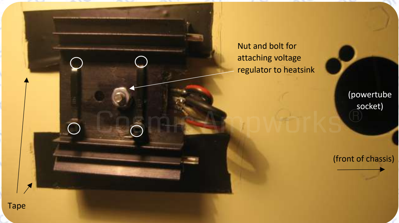
Figure 19. Drill four holes in the heatsink (locations indicated with white circles), for attaching it to the chassis with two tie wraps. Don't worry about the heat, because the heatsink has such a large capacity that its temperature will not noticeably increase.
